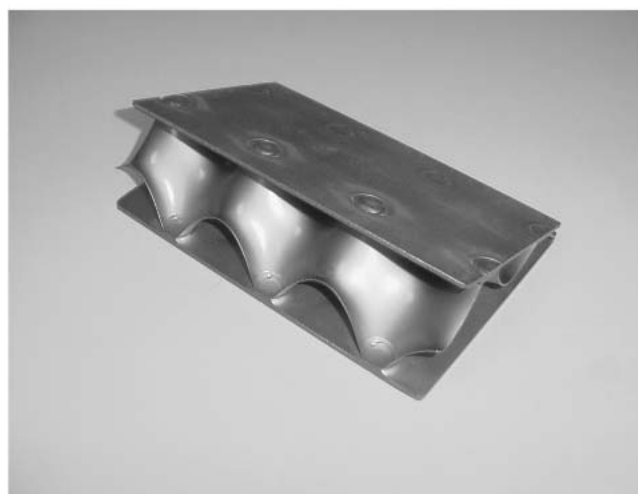
Fig. 14 Sample sections of multisheet SPF/DB truss core built by Boeing and its subsidiaries. Upper left, four-sheet welded core panel. Upper right, two-sheet stiffened panel built using yttria stop-off and gas pressure bonding in a hot isostatically pressed vessel. Lower left, circular SPF/DB using three sheets of titanium and yttria stop-off. Lower right, “dot core” built using partial penetration laser weld
