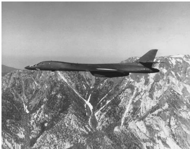
Fig. 4 Many sections of the B-1B were studied for potential SPF/DB applications.
