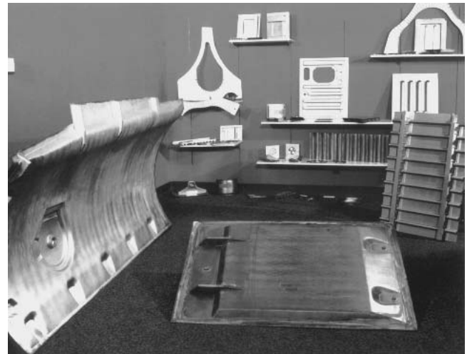
Fig. 5 Several parts were developed and prototyped using SPF/DB for the B-1B. This photograph shows many of the titanium parts that were built as demonstration and testpieces, but did not make it onto the baseline design.
